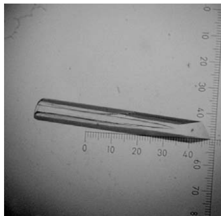
Figure 1 A crystal of EcoO109I . Its approximate dimensions are 1.0 \times 0.1 \times 0.1 mm.
